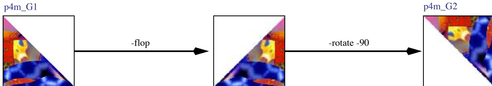
3) Generate tile\_part by composing p4m\_G1 and p4m\_G2 with Dst\_Over:
